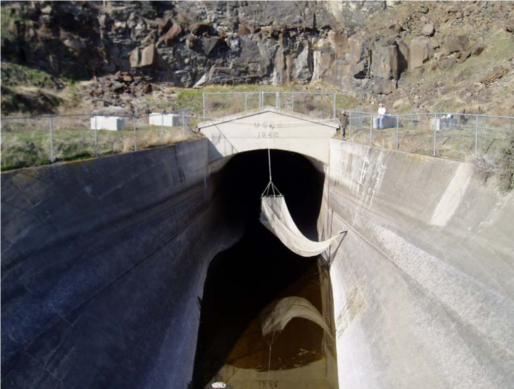
Figure 4. The trawl net (1.5 x 1.5 m opening) and rigging system used to sample fish in the west canal during the Banks Lake entrainment study 2004, 2005.
